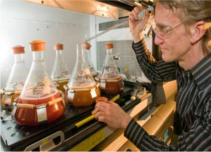
*Argonne biophysicist Philip Laible oversees the growth of new variants of photosynthetic bacteria designed to produce target bio-fuel molecules. In this culture mode, it is easy to extract cells during all phases of growth for analysis, and add chemicals (shown here) to speed growth or induce the production of target fuels.*
